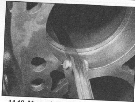
14.18 Measuring a piston ring end gap
