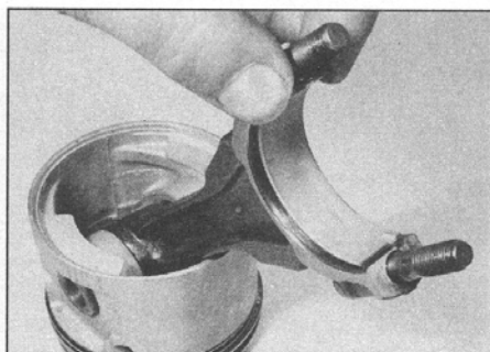
19.3a Fitting a new bearing shell to the connecting rod big-end
