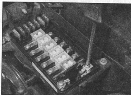
5.32b . . . then disconnect the left-hand wire from the connector plate
