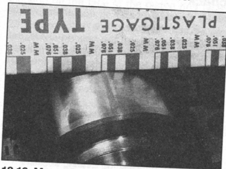
18.10 Measuring the width of the deformed Plastigauge using the card gauge
