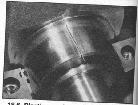
18.6 Plastigauge in place on crankshaft main bearing journal
