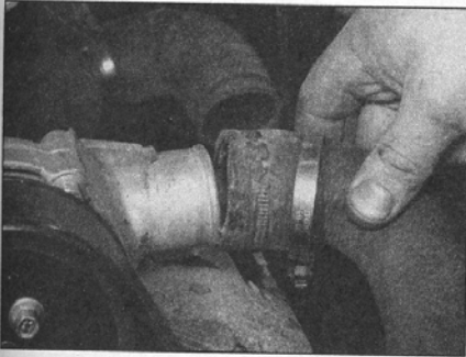
5.29a Disconnect the coolant hoses from the coolant pump . . .
