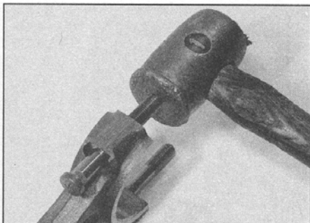
19.1 Tapping a big-end bolt from a connecting rod
