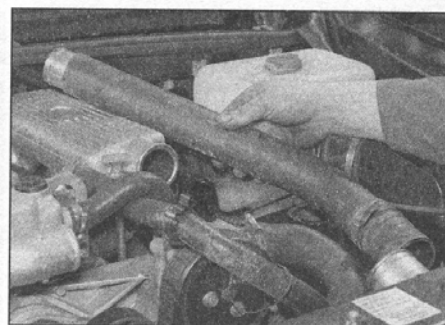
5.14b . . . and lower intercooler air trunking
