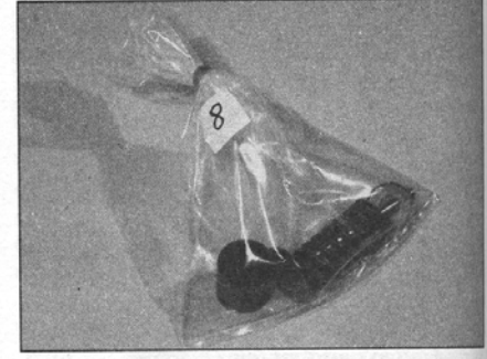
8.13 Place the valve components in a labelled polythene bag
